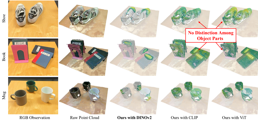
Figure 3: 3D Semantic Fields Visualization. We visualize 3D semantic fields in the scene, similar to Figure 6 in the main paper. For ours with DINOv2, object parts from different instances are highlighted consistently. For example, shoe heads, book titles, and mug handles are highlighted in these scenes. In contrast, ours with CLIP and ours with ViT fail to highlight object parts consistently. Instead, their heatmap distributes over the scene and has no distinctions among object parts.
